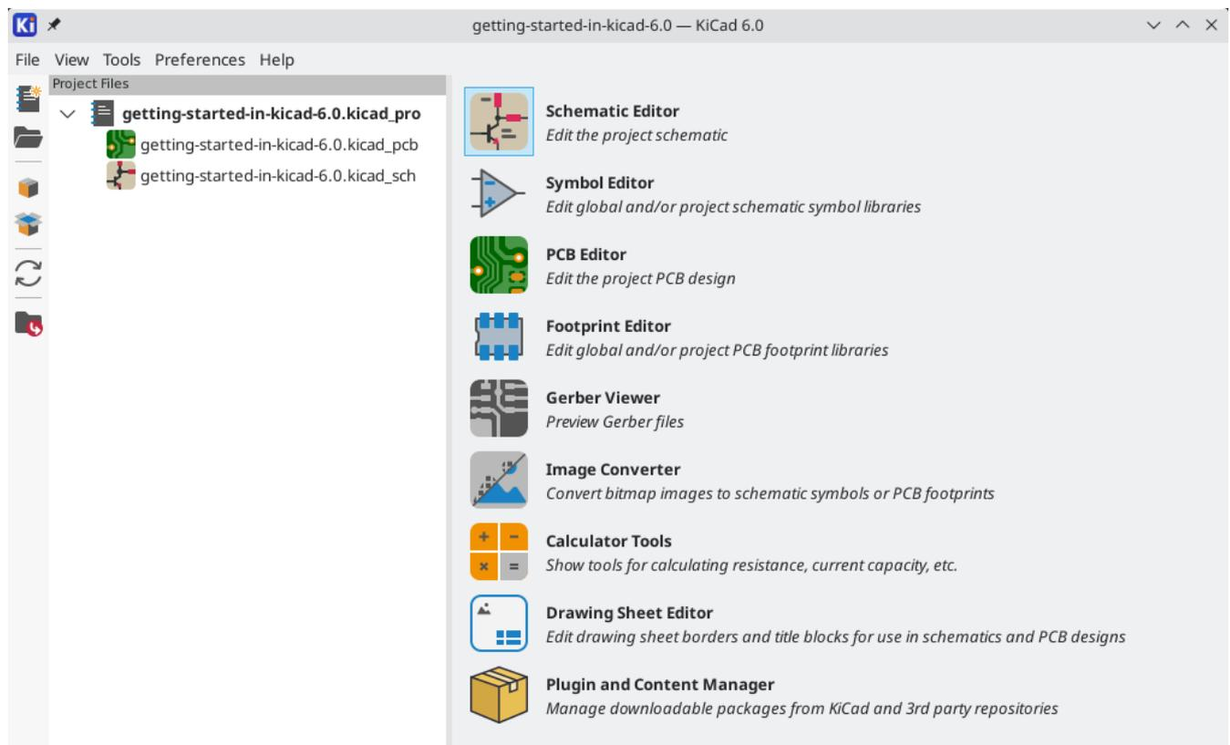
At left, the Project Files pane lists the files in the new project. There is a project file with the extension `.kicad_pro`, a schematic file with the extension `.kicad_sch`, and a board file with the extension `.kicad_pcb`. These files all share a name with your project.
