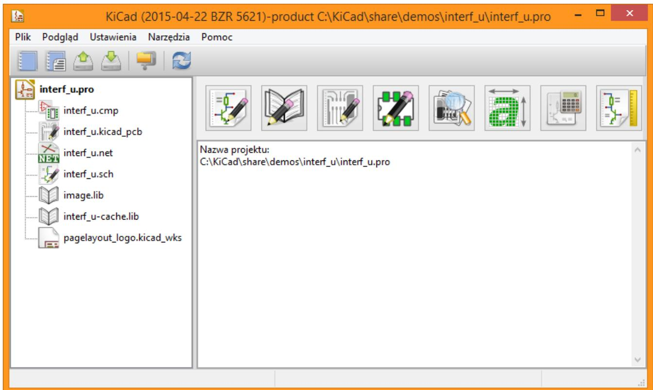
The KiCad project manager window is composed of a tree view on the left showing the files associated with the open project, and a launcher on the right containing shortcuts to the various editors and tools.
