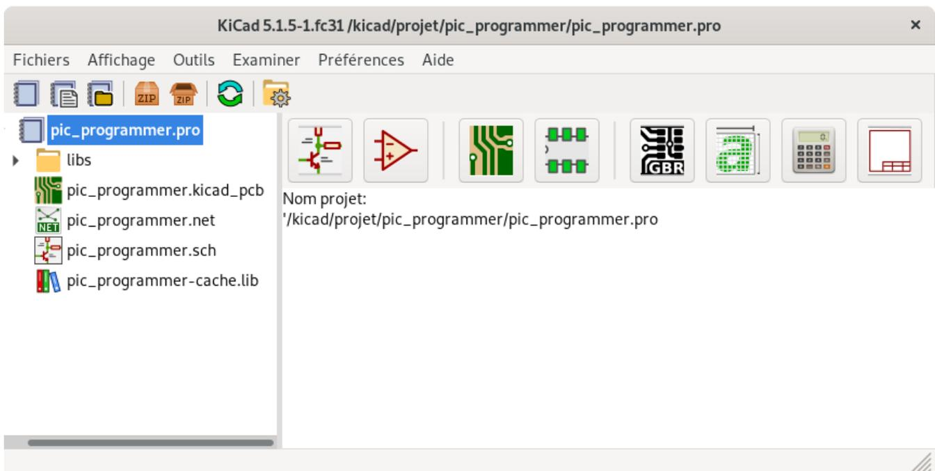
The KiCad project manager window is composed of a tree view on the left showing the files associated with the open project, and a launcher on the right containing shortcuts to the various editors and tools.
