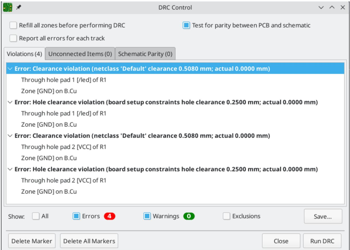
Close the DRC dialog, press **B** to refill the zone, and re-run DRC. Alternatively, check the *Refill all zones before performing DRC* checkbox and re-run DRC. All violations are fixed.
