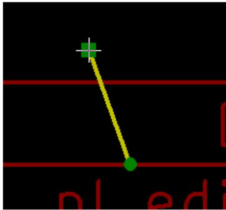
Once selected, the item, or one of its end points, can be moved by moving the mouse and placed (right clicking on the mouse).
