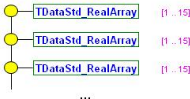
Figure 2: Allocation of data of each measurement point as arrays of double values
