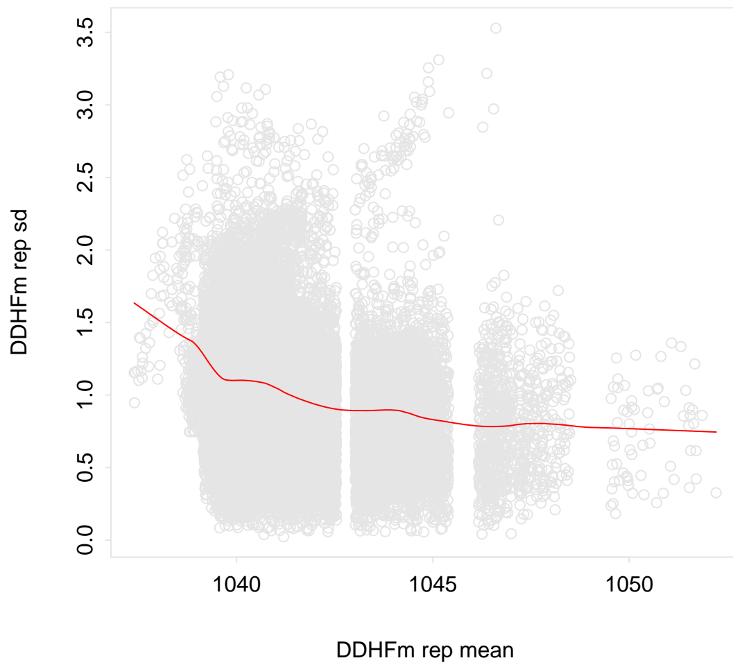
Figure 2: Replicate standard deviation versus the replicate mean for the DDHfm transformed data. Red line is best lokerns kernel smoothing fit which is not far from horizontal indicating good stabilization. The median bandwidth is 1.8.
